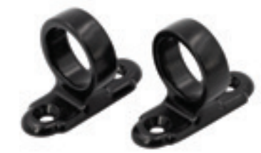
Pole Eyes Used for opening and closing the top sash. One pole eye is fitted to windows up to 479mm wide. Two are fitted on windows 480mm wide and over.
